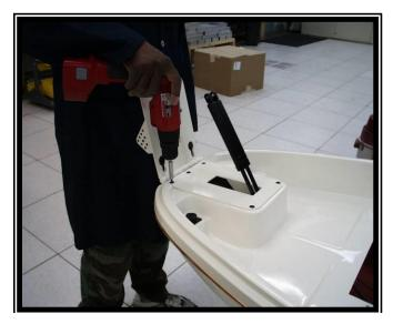
Figure 7.6.2 Removing Hinge Plate Screws on Base Chassis.
