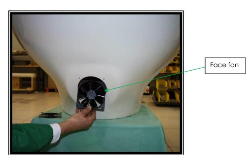
Figure 7.17.1 Inserting/Removing Face Fan Assembly.
