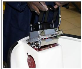
Figure 7.3.4 Removing Heater Harness.
