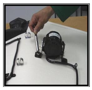
**Figure 7.9.4**Removing Flange Bolt Attaching Motors.
