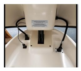
Figure 7.1.1 Releasing Electrical Connectors.
