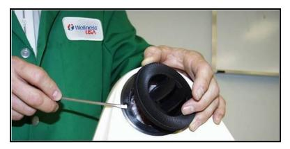
Figure 7.16.1 Removing Face Air Vent(s).
