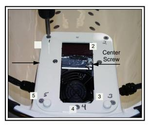
Figure 7.3.2 Removing Hinge Plate.
