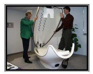
Figure 7.1.3 Removing the Hood.
